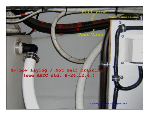
The photograph (of the port fuel tank) shows that the run, of the fill and vent lines rigged to each of the two (installed port & stbd. in the engine space) fuel tanks, are not self-draining. This situation does not comply with the provisions of **A.B.Y.C Standard H-24.12.4** "Fuel fill lines shall be self-draining and run as directly as practicable from the deck plate to the fuel tank connection and **H-24.13.7** "Tank vent systems shall be self-draining".
